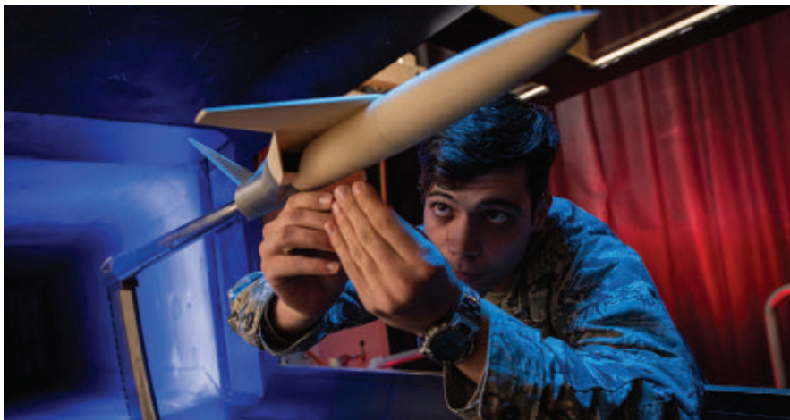
U.S. Air Force Academy Cadet Michael Higgins mounts a 3D printed model in a subsonic wind tunnel for testing at the academy in Colorado Springs, Colo.
