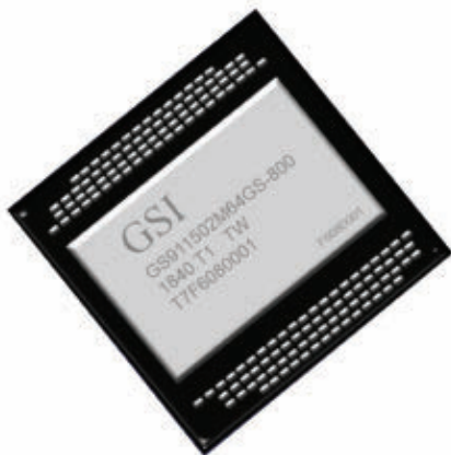
GSI Technology’s Gemini Associative Processing Unit (APU) is designed for future autonomous satellites.
