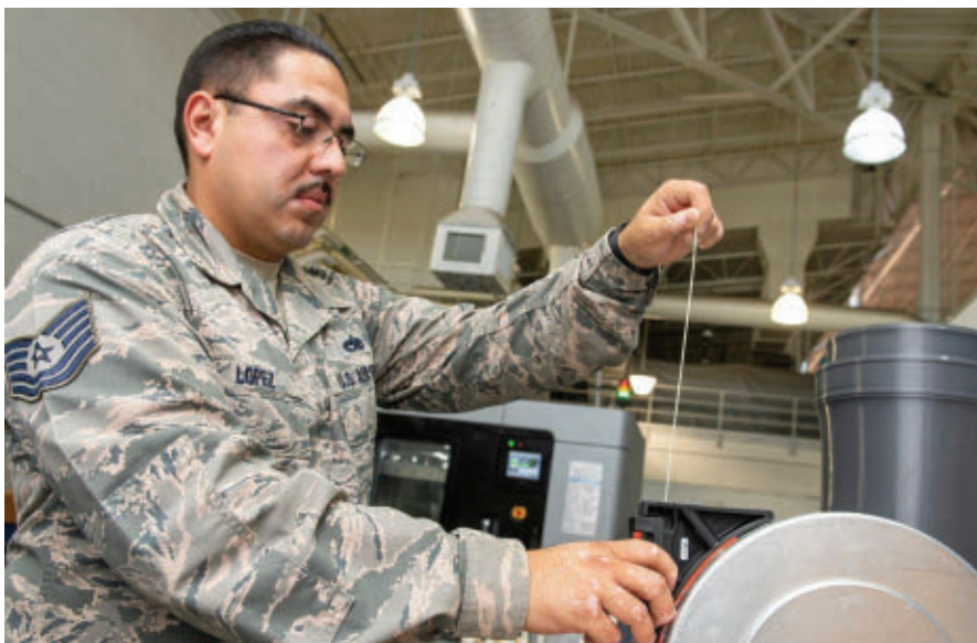
The Stratays F900 3D industrial printer is certified by the U.S. Federal Aviation Administration for use on aircraft replacement parts.
