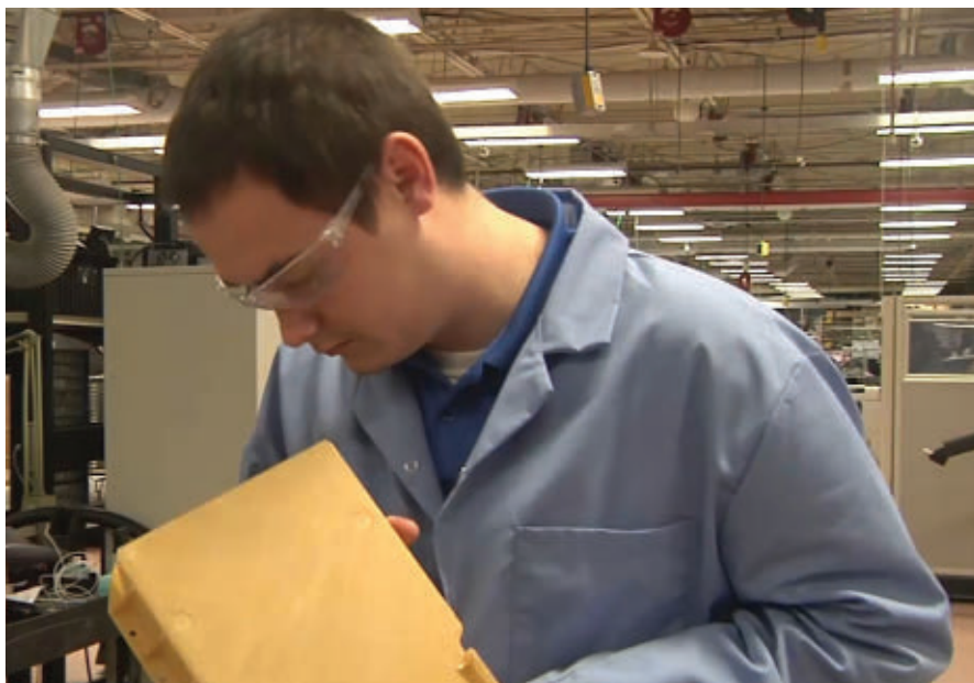
Technician at a Northrop Grumman Corp. facility in Charlottesville, Virginia, inspecting a 3D printed manifold for one of their navigation systems.
